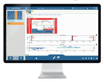
The b2 electronic GmbH PDTD60-2 Partial Discharge (PD) and Tan Delta (TD) Diagnosis System for diagnosis of medium voltage cables, rotating machinery and transformers.
