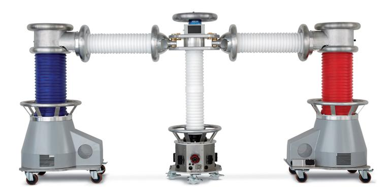
The high power HVA200 Test System is capable of testing cables up to 141 kV (Test Voltage 1.7 x U0). The smallest and lightest VLF unit of his class offers VLF (Very Low Frequency) 0.1 Hz standard testing as well as DC output voltage up to 200 kV. The HVA200 system can be upgraded with optional Tan Delta or Partial Discharge Diagnostics Systems. This space saving configuration allows the test set to be mounted on a van or trailer or can be transported in solid transport boxes (optional).
