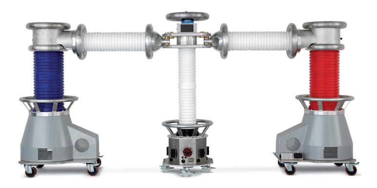
The high power HVA200 Test System is capable of testing cables up to 138 kV (Test Voltage 1.7 x U0). The HVA200 is for laboratory use or can be fitted as a mobile test laboratory into a van. The smallest and lighvtest VLF unit of his class offers VLF (Very Low Frequency) 0.1 Hz standard testing as well as DC output voltage up to 200 kV. The HVA200 system can be upgraded with optional Tan Delta or Partial Discharge Diagnostics Systems.
